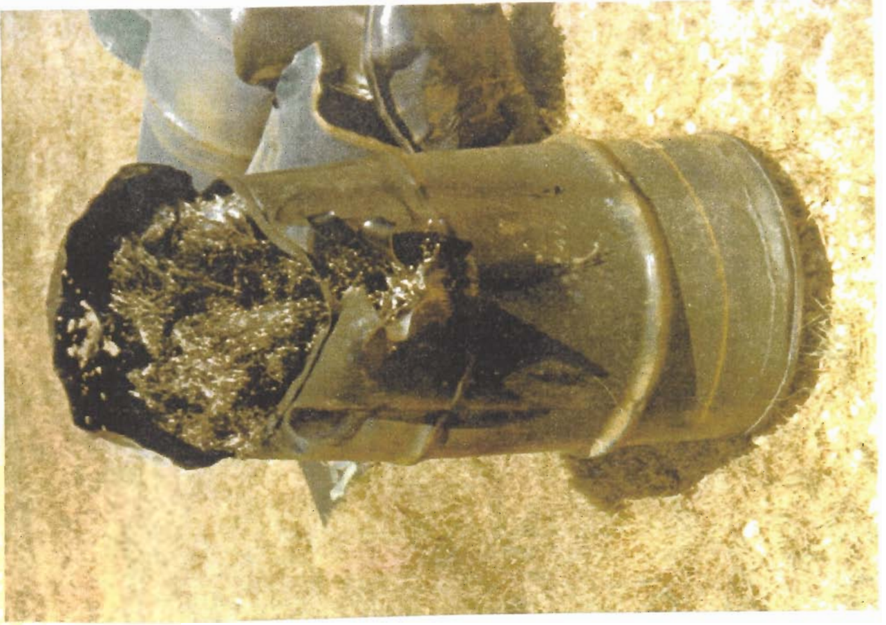
FIGURE 3. PHOTOGRAPHS ILLUSTRATING NEAR – IDENTICAL HYDRAULIC RAM RUPTURE EFFECTS OF 76 LITERS OF DIESEL FUEL IN 114-LITER DRUMS WITH AND WITHOUT EXPLOSIVE IN AFLRL SIMULATED FULL-SCALE BALLISTIC TEST
