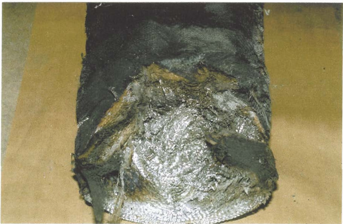
Figure 14. DETO-STOP from Vapor-Space Ballistic Test; 10 Gallons
