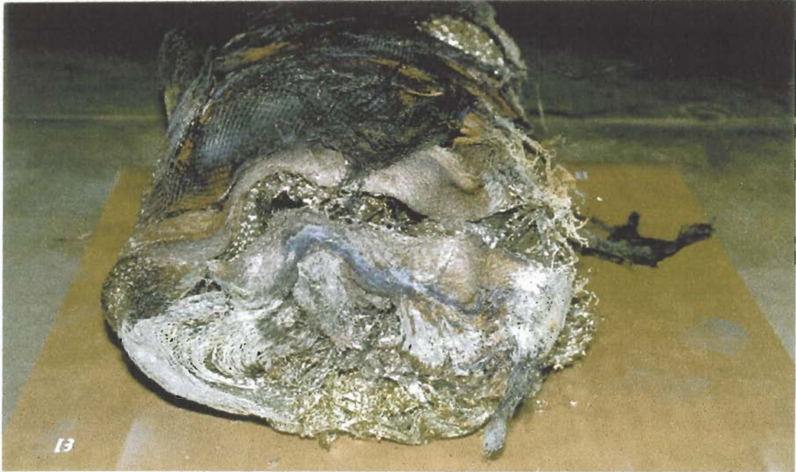
Figure 15. DETO-STOP from Liquid Level Ballistic Test; 20 Gallons
